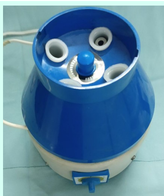
Figure 1: Table top centrifuge machine and subjected to centrifugation for 10 min at 3000 rpm.
